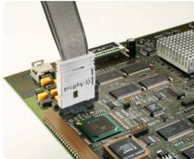
E5346A 34-channel Mictor connector probe
