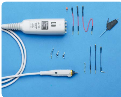
Agilent 1156A active probe with accessories
