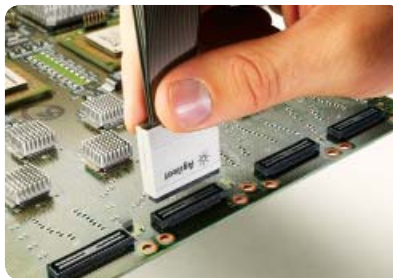
E5385A 34-channel Samtec connector probe
