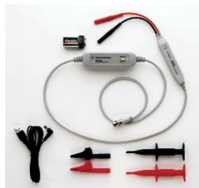
N2792A 200 MHz, 20 V differential probe
