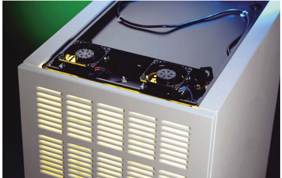
Extractor fan installed in rack
