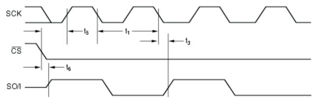
Figure 10. Output Data Timing Diagram
