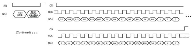
Figure 4. READ followed by WRITE Command to Configuration Register
