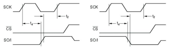
Figure 12. Input Data Timing Diagram
