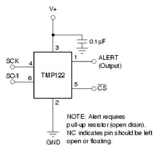
**Figure 1. Typical Connections**
