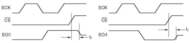
Figure 11. High Impedance Output Timing Diagram
