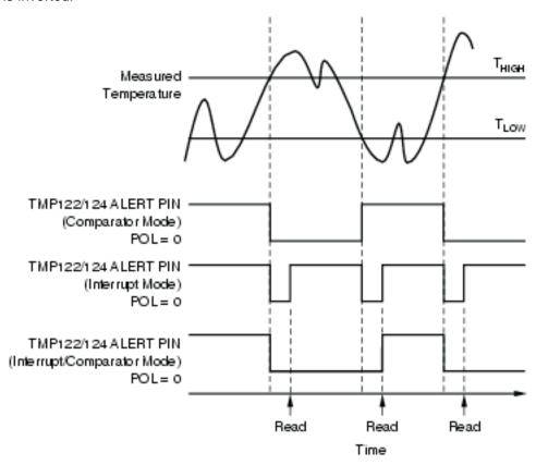
Figure 8. ALERT Output Transfer Function Diagrams
