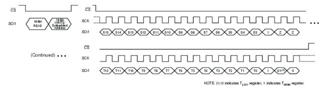
Figure 3. READ followed by WRITE Command to T<sub>LOW</sub>/T<sub>HIGH</sub> Register
