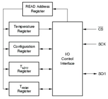
Figure 7. Internal Register Structure
