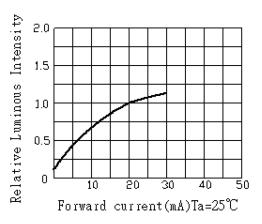
Luminous Intensity vs.Forward current
