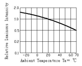
Luminous Intensity vs. Ambient Temperature
