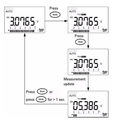
Figure 3-2 Data hold mode operation
