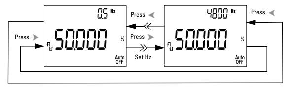
Figure 3-11 Frequency adjustment for square wave output
