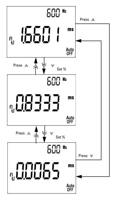
Figure 3-13 Pulse width adjustment for square wave
