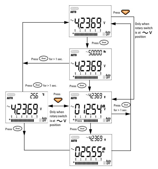
Figure 3-5 dBm/dBV display mode operation
