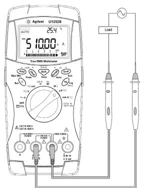
Figure 2-3 Measuring  $\mu A$  and mA current
