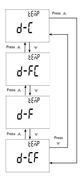
Figure 4-6 Temperature unit setup
