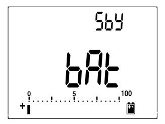
Figure 5-1 Battery capacity display as trickle
