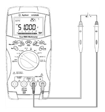
Figure 2-2 Measuring DC voltage
