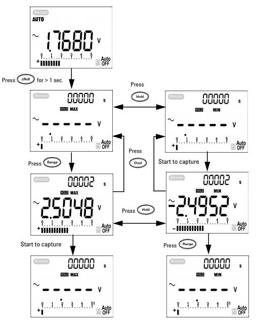
Figure 3-6 1 ms peak hold mode operation
