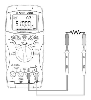
Figure 2-7 Measuring resistance
