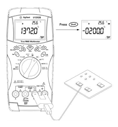
Figure 2-12 Surface temperature measurement
