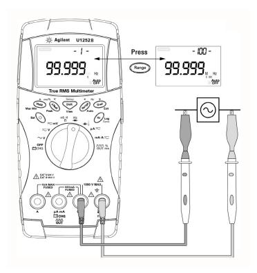
Figure 2-6 Measuring frequency
