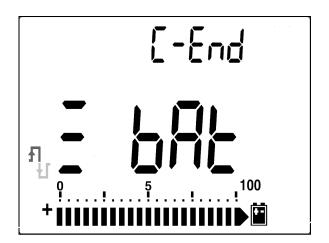
Figure 5-5 Charge end and trickle state
