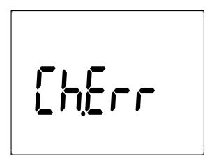
Figure 2-14 Charge terminal alert
