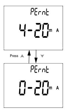
Figure 4-8 % scale readout setup
