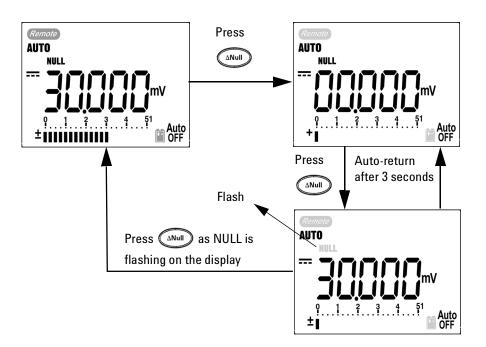
Figure 3-4 Null (relative) mode operation
