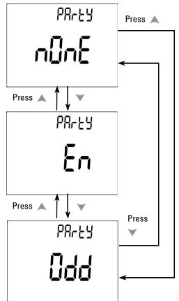
Figure 4-12 Parity check setup
