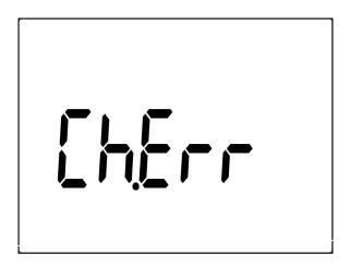
Figure 6-3 Charge terminal alert
