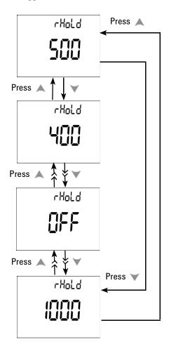
Figure 4-1 Data hold/Refresh hold setup
