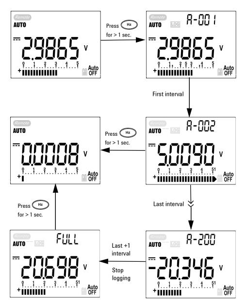
Figure 3-9 Interval (Automatic) logging mode operation
