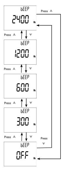
Figure 4-9 Beep frequency setup
