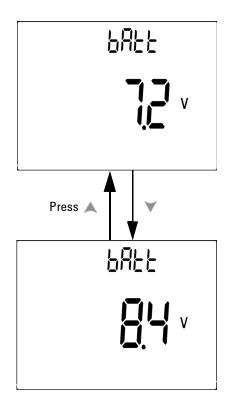
Figure 4-17 Battery voltage selection
