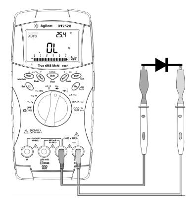
Figure 2-11 Measuring reverse bias of diode
