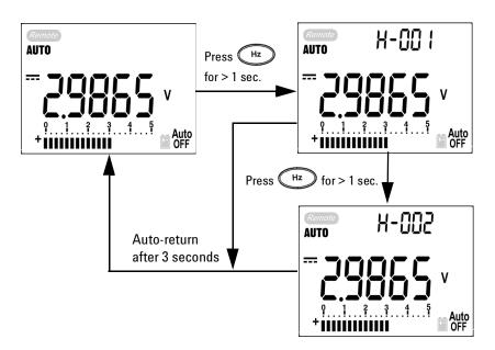
Figure 3-7 Hand (Manual) logging mode operation
