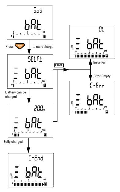
Figure 5-6 Battery charging procedures
