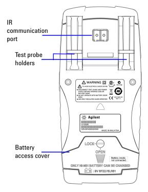
Figure 1-2 Rear panel of U1252B
