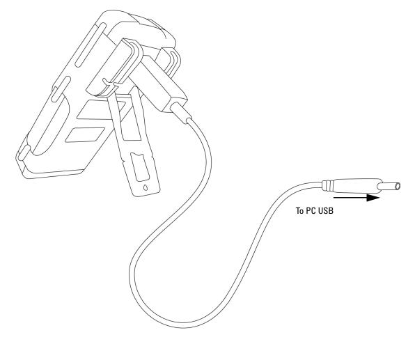
Figure 3-14 Cable connection for remote communication
