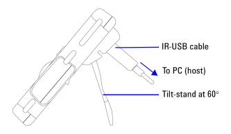
To adjust the meter to a  $30^{\circ}$  standing position, bend the tip of the stand so that it is parallel to the ground before pulling the stand outwards to its maximum reach.
