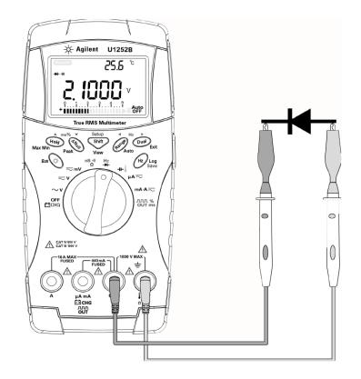
Figure 2-10 Measuring forward bias of diode
