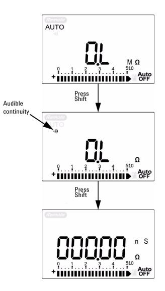
Figure 2-8 Audible continuity, conductance and resistance test.
