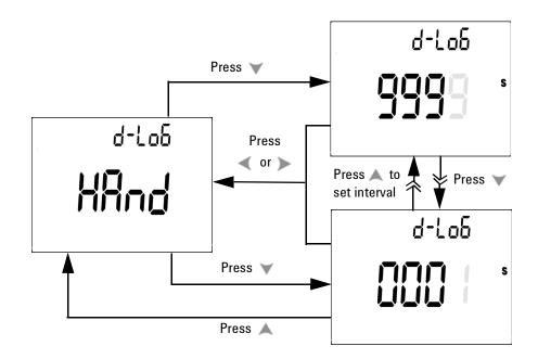
Figure 4-2 Data logging setup
