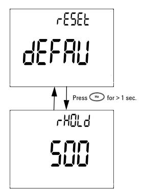
Figure 4-16 Reset setup
