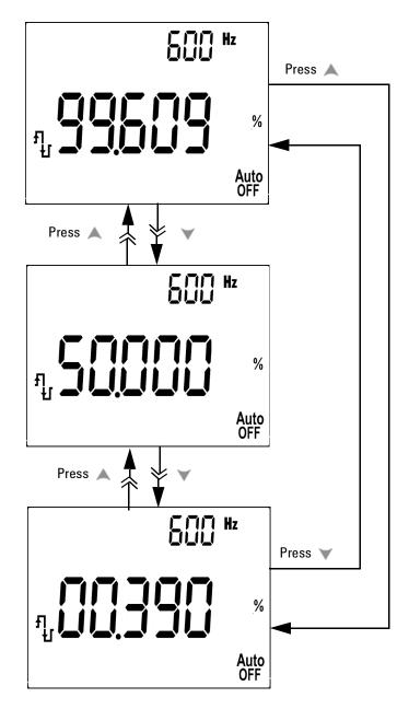
Figure 3-12 Duty cycle adjustment for square wave output
