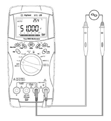
Figure 2-1 Measuring AC voltage
