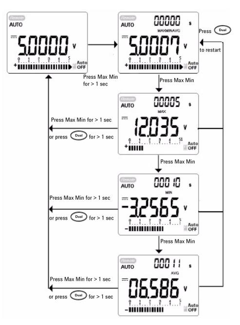
Figure 3-1 Dynamic recording mode operation
