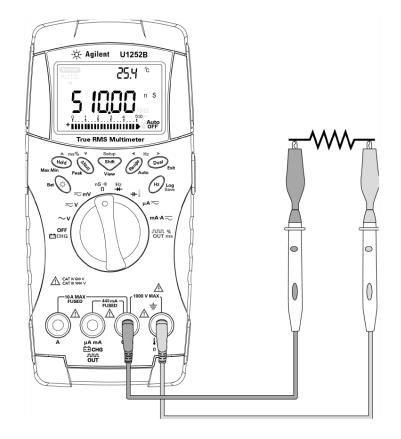
Figure 2-9 Conductance measurement
