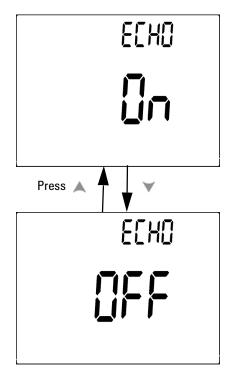
Figure 4-14 Echo mode setup for remote control
