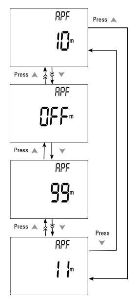
Figure 4-7 Auto power saving setup
