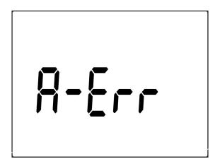
Figure 2-13 Input terminal warning
