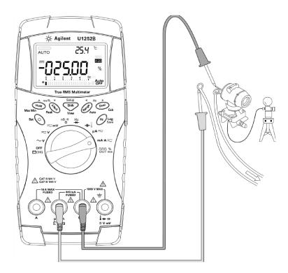
Figure 2-4 Measuring scale of 4-20 mA
