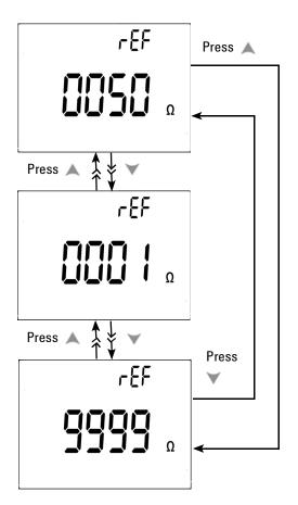
Figure 4-4 Reference impedance for dBm measurement setup
