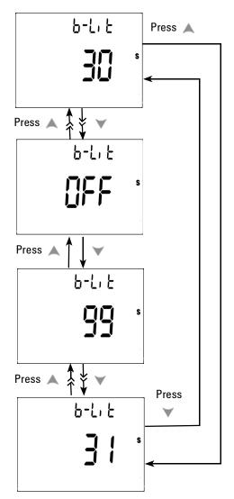
Figure 4-10 Backlit timer setup
