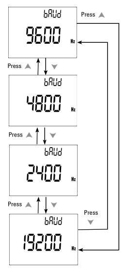
Figure 4-11 Baud rate setup remote control
