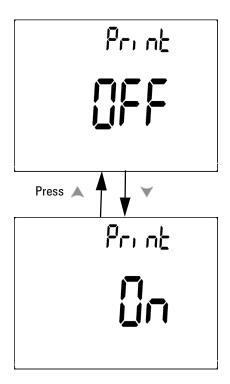
Figure 4-15 Print mode setup for remote control
