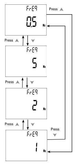
Figure 4-5 Minimum frequency setup
