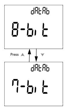
Figure 4-13 Data bit setup for remote control
