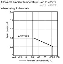
1.-(2) Load current vs. ambient temperature characteristics
