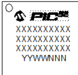
144-Lead TFBGA (7x7x1.02 mm)
