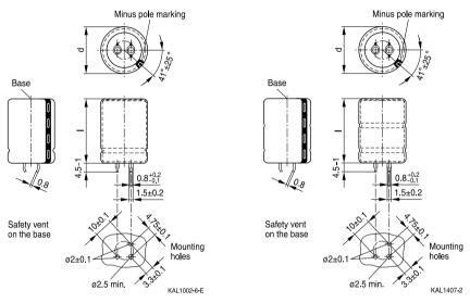
Snap-in capacitors are available with 3 terminals (length (4.5 - 1) mm). PET insulation is marked with label "PET" on the sleeve.
