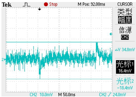
15. Load transient response (IL=10-350-10mA)
