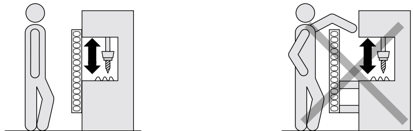
Figure 8: Representation of the accessibility of ESPE by reaching over. Left: Protective field that cannot be reached over. Right: Protective field that can be reached over.
