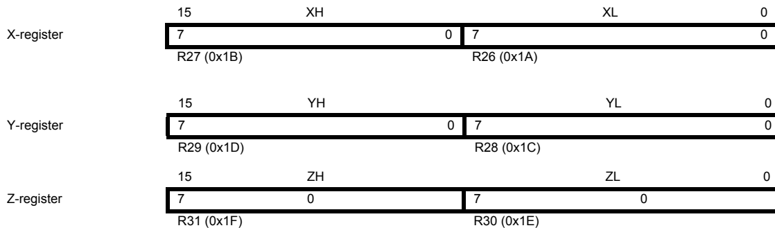
Figure 7-3. The X-, Y-, and Z-registers.
