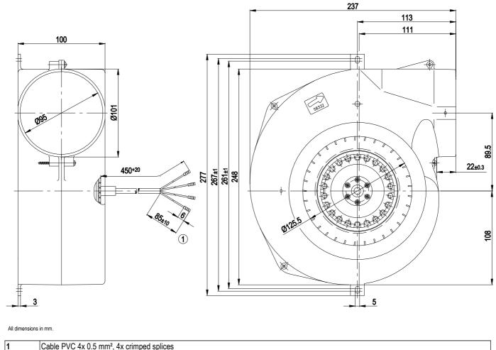
Cable PVC 4x 0.5 mm<sup>2</sup>, 4x crimped splices
