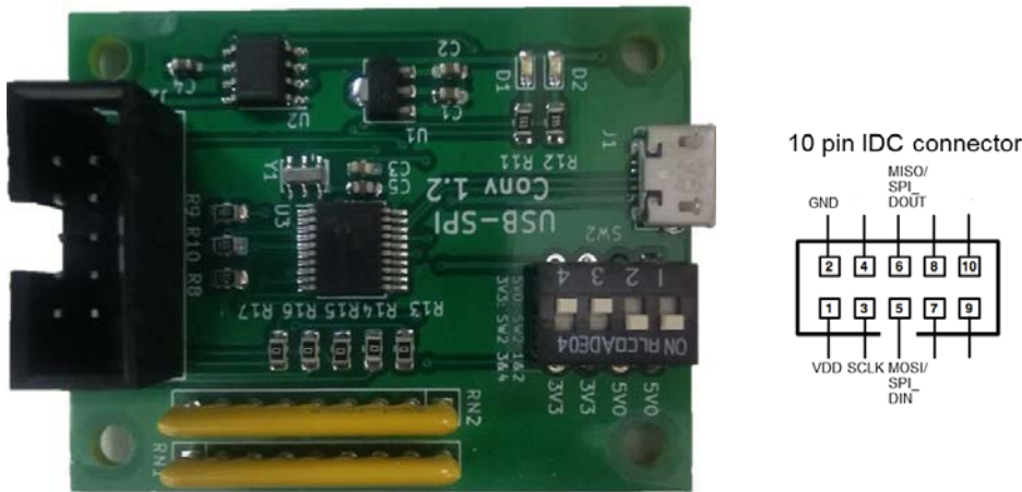
Figure 9: HEDS-9930PRGEVB USB-to-SPI Programmer Kit Schematic
