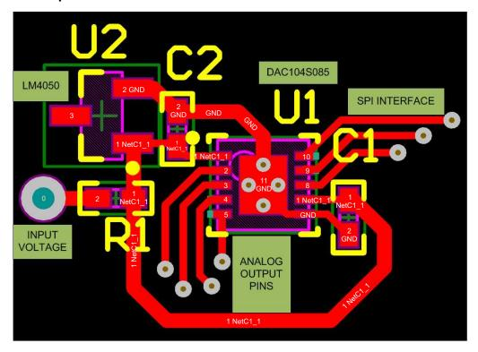
Figure 39. DAC104S085 Layout Example
