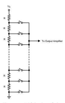
Figure 26. DAC Resistor String
