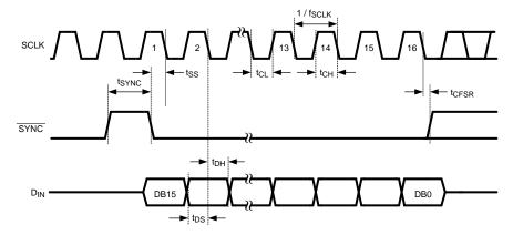
Figure 1. Serial Timing Diagram
