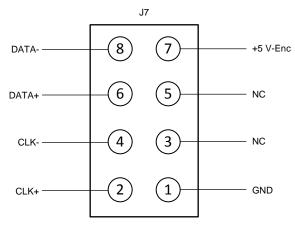
Figure 11. Abs-Enc-1 (J7) Pinout on TIDM-1008 Board
