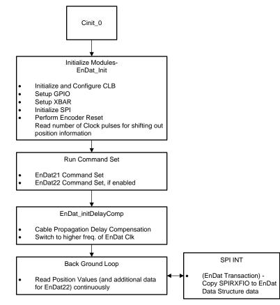
Figure 13. Software Flow Diagram for Example Project PM\_endat22\_BasicPosAcc\_DelComp
