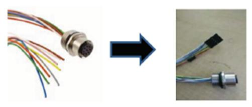
Figure 10. Adapter to Connect Heidenhain Cable to TIDM-1008 Board
