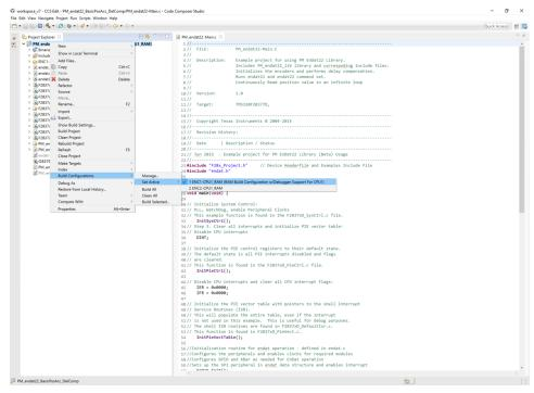
Figure 8. Selecting F2837x\_RAM Configuration
