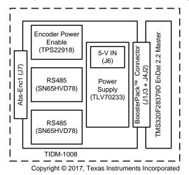
Figure 1. TIDM-1008 Hardware Blocks and Connectors
