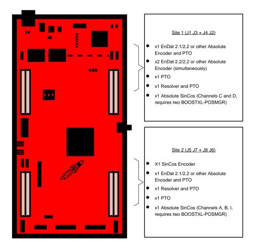
Figure 3. TIDM-1008 Board and BOOSTXL-POSMGR Encoder Support
