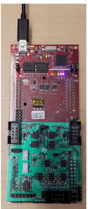
Figure 9. TIDM-1008 Board Connected to Site Two of LaunchPad™
