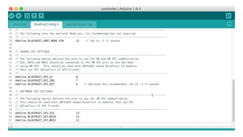
For all the example code, we have at the top of the sketch a few different ways you can communicate with the Bluefruit LE: hardware serial, software serial, hardware SPI and software SPI.
