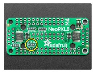
Locate the  ${\bf n0}$  selector pads on the FeatherWing and use an X-Acto knife or small file to  ${\bf cut}$  the trace between  ${\bf n0}$  and SCK.
