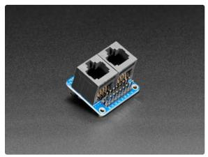
In either case, the NeoPixel headers mount on the *FLAT SIDE* of the NeoPXL8 Friend — the side with NO COMPONENTS — and are soldered on the *component side*. The breadboarding pins are done the OPPOSITE way — install from the component side, solder on the flat side.
