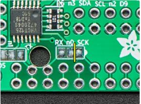
Solder a short piece of insulated solid-core wire between the now-isolated **n0** surface pad and the last through-hole via in this row.
