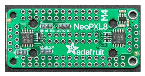
Let's refer to NeoPXL8's eight outputs as "0" through "7," sequentially. Outputs 4, 5, 6 and 7 are fixed to specific Feather pins (13, 12, 11 and 10) and *cannot* be changed, period. Outputs 0, 1, 2, and 3 offer a "this" or "that" choice.
