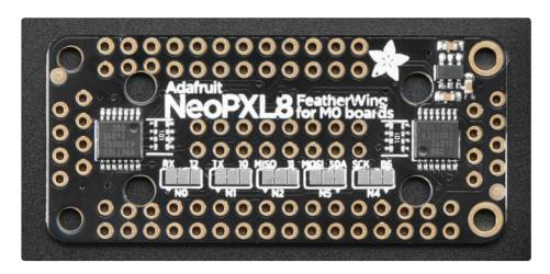
Let's refer to NeoPXL8's eight outputs as "0" through "7," sequentially. Outputs 3, 6 and 7 are fixed to specific Feather pins (13, A4, A3) and *cannot* be changed, period. Outputs 0, 1, 2, 4 and 5 offer a "this" or "that" choice.
