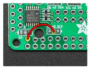
If you'll be using the RJ-45 connections for pixels, make sure this wire clears the mounting hole in the board.
