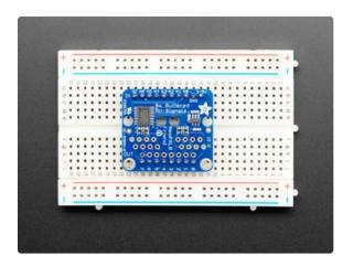
A third option is to install header pins on the NeoPixel outputs, so both the "ins" and "outs" are breadboardable...this may be useful for certain prototyping tasks.
