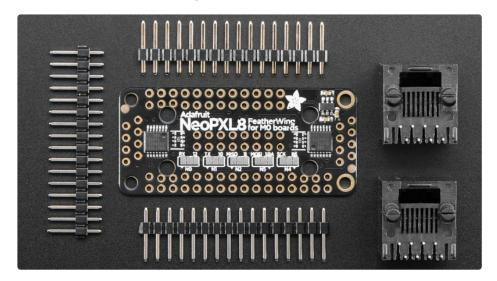
For NeoPixel projects starting with one of our **Feather M0** or **M4** board variants, a **NeoPXL8 FeatherWing** can simplify and make sense of the wiring...the boards are designed to be stacked. **Some soldering and "maker skills" are required.**
