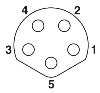
Pin assignment of M8 socket, 5-pos., B-coded
