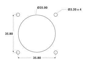
When mounted this way the panel acts as the bezel and no separate bezel is needed. M3 machine screws are recommended.
