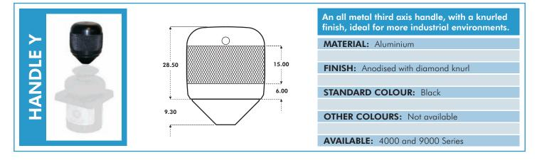
The total throw of all third axis handles is  $55^{\circ}$  (+/- 27.5 degrees). As standard the polarity of all the handles is incrementing when turned clockwise.
