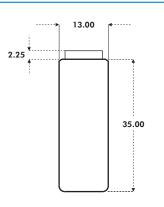
A soft touch push button handle, using the Apem 9633 Series switch.
