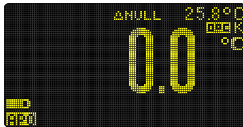
Figure 2-30 Temperature measurement without ambient compensation
