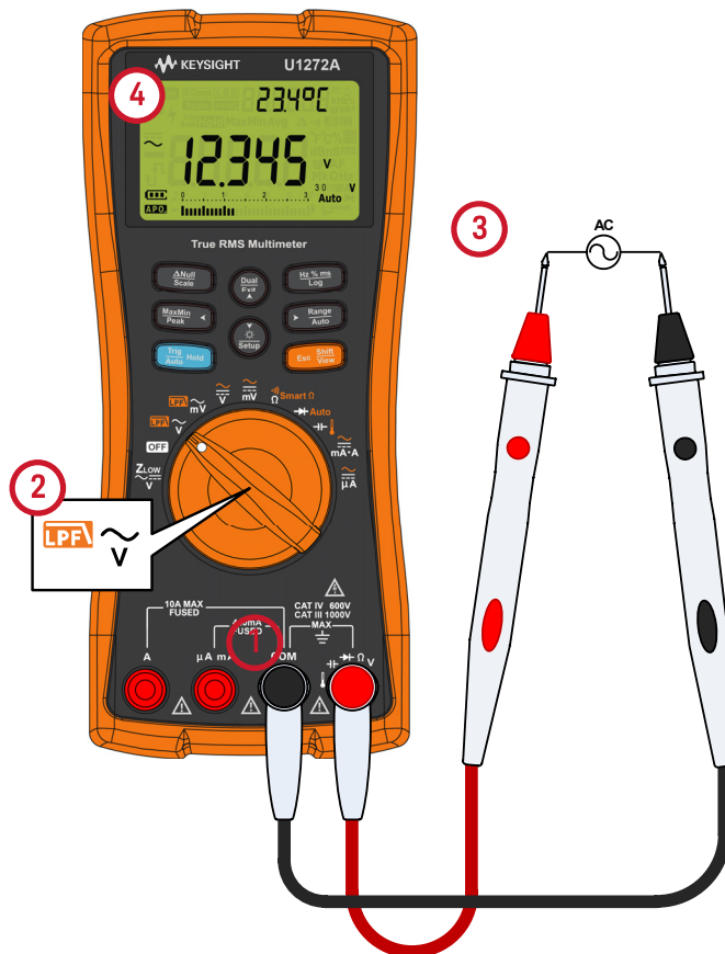
Figure 2-2 Measuring AC voltage
