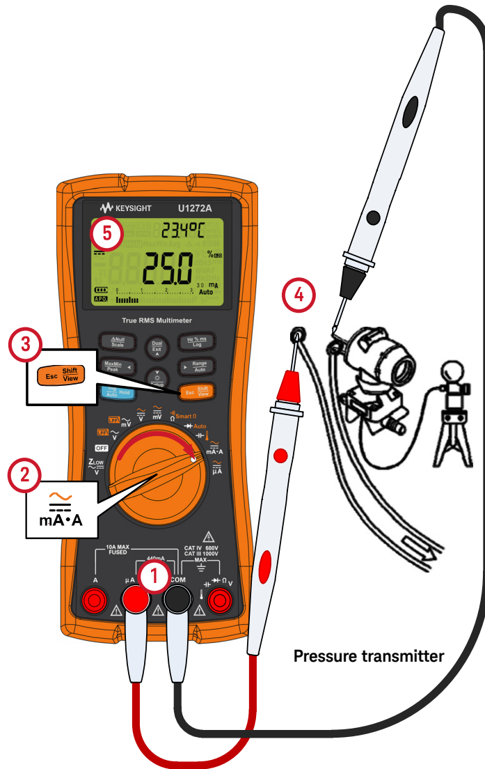
Figure 2-36 Measuring DC current using the 0-20 mA % scale
