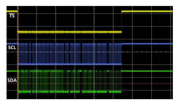
Figure 7-1. Example for TS Line Indication and Following Read Operation
