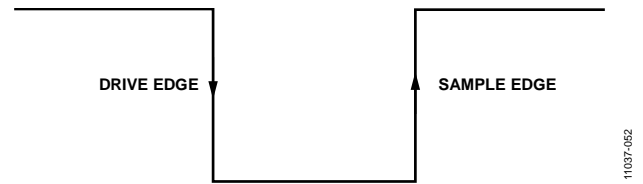
Figure 38. SPI Mode 3 SCLK Edges
