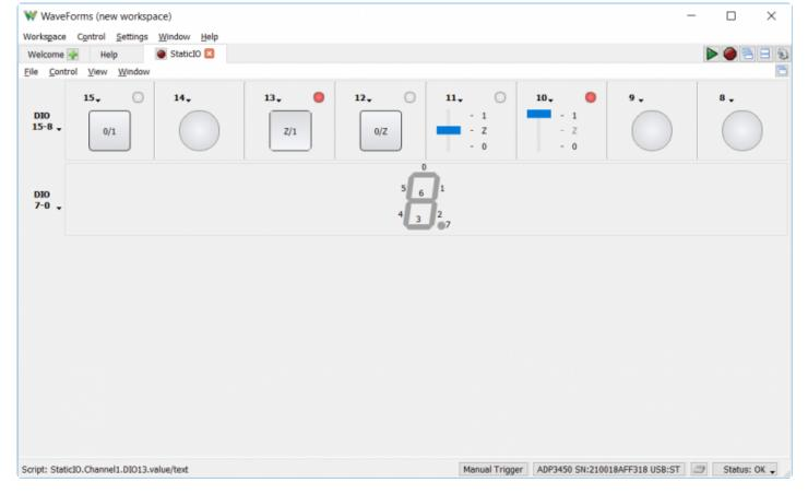
The Analog Discovery Pro (ADP3450/ADP3250) can be used with WaveForms' Static I/O instrument to emulate a variety of user input/output devices on the digital input/output pins. Virtual LEDs, buttons, switches, sliders, and displays can be assigned to specific digital I/O pins, and interacted with within the WaveForms user interface.
