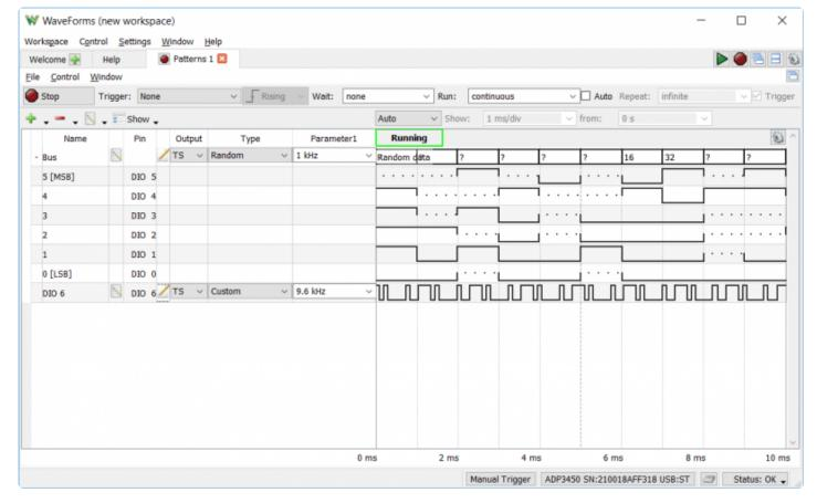
The Analog Discovery Pro (ADP3450/ADP3250) can be used with WaveForms' "Patterns" instrument to generate logic signal sequences on the digital input/output pins. Each channel can be configured to be push/pull, open drain, open source, or three-state logic and set to generate Clock, pulse, random or custom patterns.
