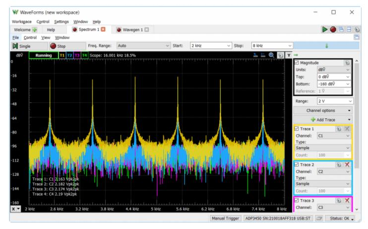
The Analog Discovery Pro (ADP3450/ADP3250) can be used with WaveForms' "Spectrum" instrument to view the power of frequency-domain components of analog signals captured on the analog input channels.
