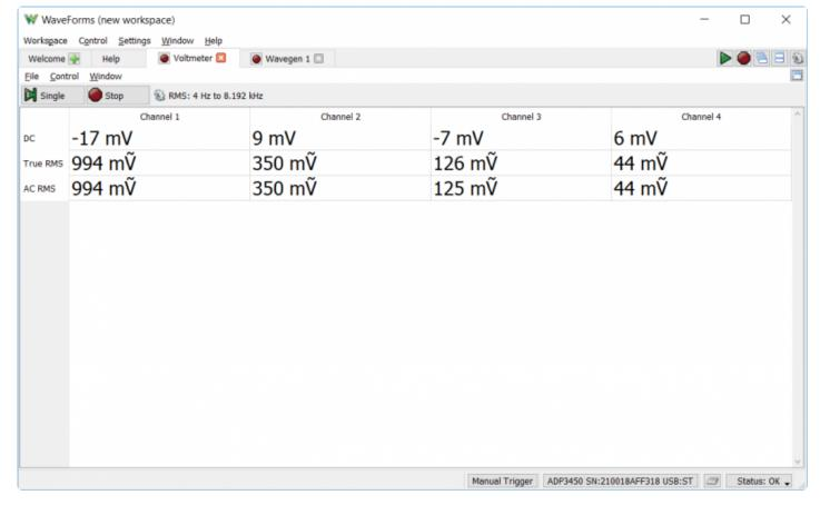
The Analog Discovery Pro (ADP3450/ADP3250)'s analog inputs can be used with WaveForms' Voltmeter instrument to act as a simple 4 channel voltmeter. DC voltages, AC RMS voltages, and True RMS voltages can be viewed for each Scope channel.
