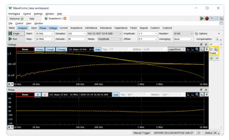
The Analog Discovery Pro (ADP3450/ADP3250) can be used with WaveForms' "Impedance" instrument to view a wide variety of frequency response characteristics of a circuit under test. Input, Phase, Voltage, Current, Impedance, Admittance, Inductance, Factor, and Nyquist plots are all available. In addition, Custom plots can be used to present the results of a wide variety of different mathematical operations on buffered data.
