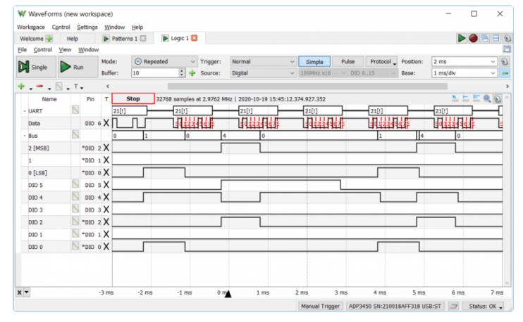
The Analog Discovery Pro (ADP3450/ADP3250) can be used with WaveForms' "Logic" instrument to act as a Logic Analyzer. When used this way, the 16 digital input/output channels are configured to capture high/low logic states on connected pins at a sample rate of up to 125 MS/s (). These channels are capable of interfacing with 3.3V and 1.2V logic signals, and when configured as inputs are tolerant of voltages of up to 5V.
