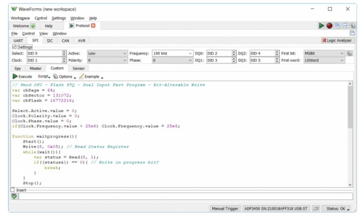
The Analog Discovery Pro (ADP3450/ADP3250) can be used with WaveForms' "Protocol" instrument to work with common communications protocols. UART, SPI, I2C, and CAN transactions can be received, transmitted, and/or spied upon by the Analog Discovery Pro using any of the 16 digital input/output channels at a sample rate of 100 MS/s.(). AVR microcontrollers can be programmed through the instrument as well.
