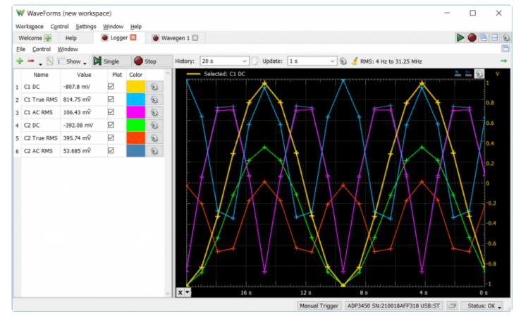
The Analog Discovery Pro (ADP3450/ADP3250) can be used with WaveForms' "Logger" instrument in order to capture large buffers of analog input data on the 4 Scope channels.
