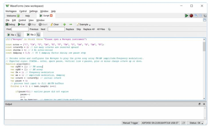
Each of WaveForms' instruments can be controlled through scripts within the WaveForms application itself. WaveForms' "Script" instrument allows the user to write and run JavaScript code that can control the rest of the application through an extensive APL(). This allows the user to configure and run many instruments at the same time, in an easily repeatable way.
