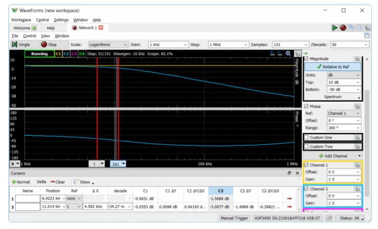
The Analog Discovery Pro (ADP3450/ADP3250) can be used with WaveForms' "Network" instrument to view the amplitude and phase response of a circuit under test. Nichols and Nyquist plots can also be viewed with this instrument.
