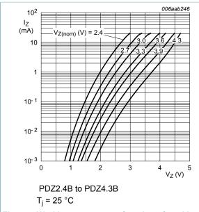
Fig. 5. Working current as a function of working voltage; typical values
