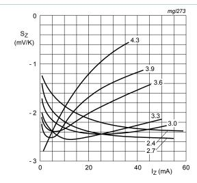
PDZ2.4B to PDZ4.3B  $T_i = 25 \,^{\circ}\text{C}$  to 150  $^{\circ}\text{C}$
