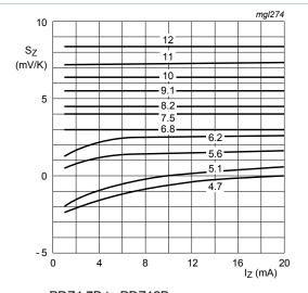
PDZ4.7B to PDZ12B  $T_j = 25 \,^{\circ}\text{C}$  to 150  $^{\circ}\text{C}$
