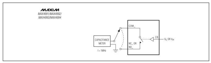
Figure 3. Channel Off-/On-Capacitance
