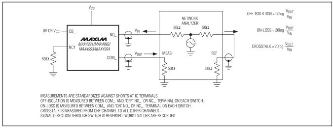
Figure 2. On-Loss, Off-Isolation, and Crosstalk
