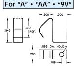
Tape and Reel Spec's:32mm wide; 12mm pitch; 13 inch reel (400 pieces per reel)
