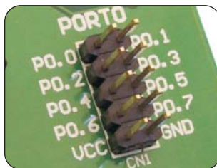
Figure 35 PORT P0 connection
