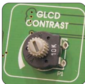
Figure 20 GLCD contrast adjustment potentiometer
