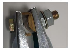
The **POINTS OF CONTACT** must be in Brass, with a shape like in the picture.
