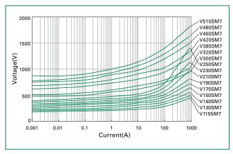
NOTE: If pulse ratings are exceeded, a shift of  $V_{N(DC)}$  (at specified current) of more than ±10% could result. This type of shift, which normally results in a decrease of  $V_{N(DC)}$ , may result in the device not meeting the original published specifications, but it does not prevent the device from continuing to function, and to provide ample protection.
