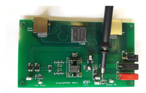
Figure 2: Output Ripple Measurement
