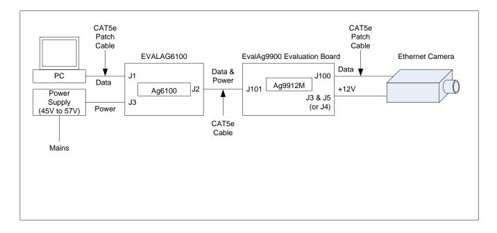
Figure 4: Example set-up
