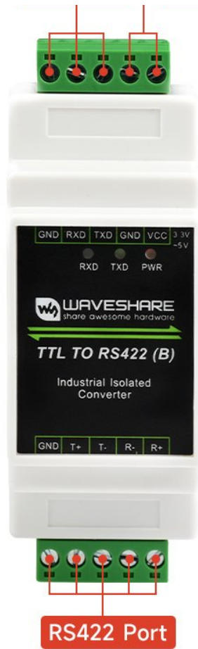
Built-in 120R selection header, enabled by default
