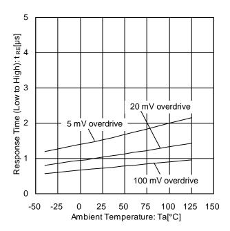
Figure 36. Response Time (Low to High) vs Ambient Temperature ( $V_{CC}$ =5 V, $V_{RL}$ =5 V, $R_{L}$ =5.1 k $\Omega$ )
