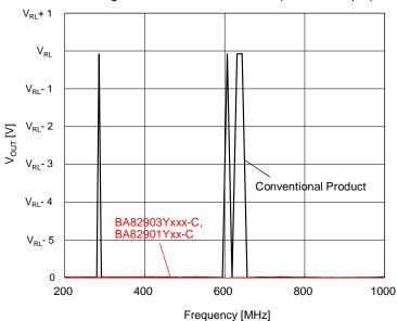
Figure 43. EMI Characteristics (L Level Output)
