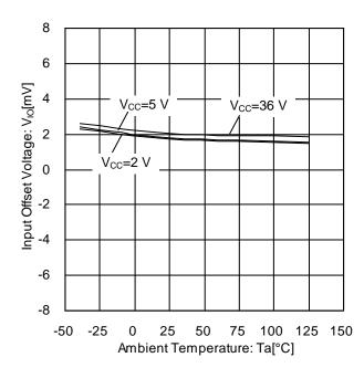
Figure 27. Input Offset Voltage vs Ambient Temperature
