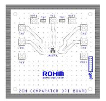
Figure 44. EMI Evaluation Board (BA82903Yxxx-C)
