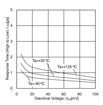
Figure 18. Response Time (High to Low) vs Overdrive Voltage ( $V_{CC}$ =5 V, $V_{RL}$ =5 V, $R_L$ =5.1 k $\Omega$ )
