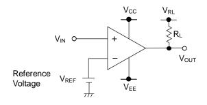
While the input voltage  $(V_{IN})$  is higher than the reference voltage, the output voltage remains high. In case the input voltage becomes lower than the reference voltage, the output voltage will turn low.
