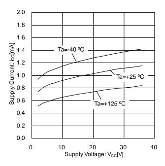
Figure 20. Supply Current vs Supply Voltage
