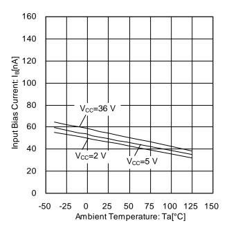
Figure 29. Input Bias Current vs Ambient Temperature
