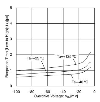
Figure 35. Response Time (Low to High) vs Overdrive Voltage ( $V_{CC}$ =5 V, $V_{RL}$ =5 V, $V_{RL}$ =5.1  $k\Omega$ )
