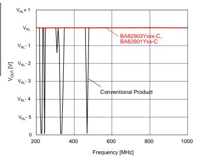
Figure 42. EMI Characteristics (H Level Output)
