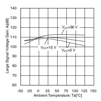
Figure 14. Large Signal Voltage Gain vs Ambient Temperature
