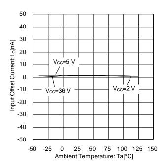
Figure 31. Input Offset Current vs Ambient Temperature
