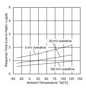
Figure 17. Response Time (Low to High) vs Ambient Temperature ( $V_{CC}$ =5  $V_{VRL}$ =5  $V_{RL}$ =5.1  $k\Omega$ )
