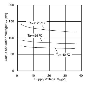
Figure 3. Output Saturation Voltage vs Supply Voltage (I<sub>SINK</sub>=4 mA)
