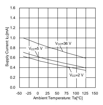
Figure 2. Supply Current vs Ambient Temperature
