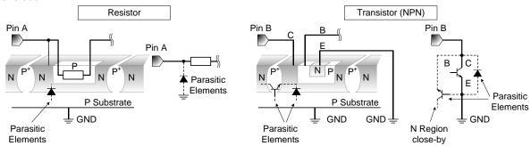
Figure 49. Example of Monolithic IC Structure
