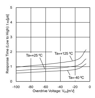
Figure 16. Response Time (Low to High) vs Overdrive Voltage  $(V_{CC}=5 \text{ V}, V_{RL}=5 \text{ V}, R_L=5.1 \text{ k}\Omega)$
