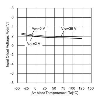
Figure 8. Input Offset Voltage vs Ambient Temperature
