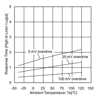
Figure 38. Response Time (High to Low) vs Ambient Temperature ( $V_{CC}=5 \text{ V}, V_{RL}=5 \text{ V}, R_L=5.1 \text{ k}\Omega$ )
