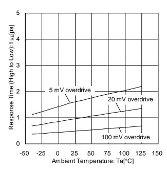
Figure 19. Response Time (High to Low) vs Ambient Temperature  $(V_{CC}=5 \text{ V}, V_{RL}=5 \text{ V}, R_L=5.1 \text{ k}\Omega)$
