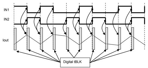
The Digital tBLK is inserted at the beginning of each charge period of the constant current chopping, and also when either of INA1, INA2, INB1, or INB2 is switched.
