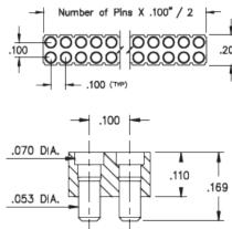
Shell Plating: 10 μ" Gold over 100 μ" Nickel Packaging: Packaged in Bulk
