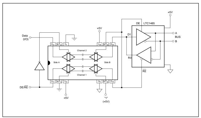
FIGURE 2. Isolated RS-485 Interface.
