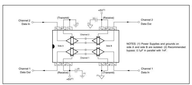
FIGURE 1. Basic Operation Diagram.
