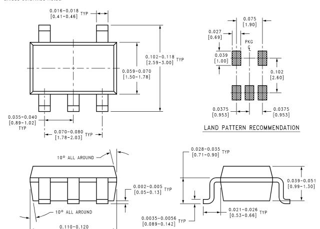
5-Pin SOT Package Order Number LMC7101AIM5, LMC7101AIM5X, LMC7101BIM5 or LMC7101BIM5X **NS Package Number MA05A**
