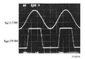
FIGURE 2. A ±7.5V Input Signal Greatly Exceeds the 3V Supply in *Figure 3* Causing No Phase Inversion Due to R<sub>I</sub>
