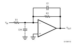
FIGURE 5. Cancelling the Effect of Input Capacitance
