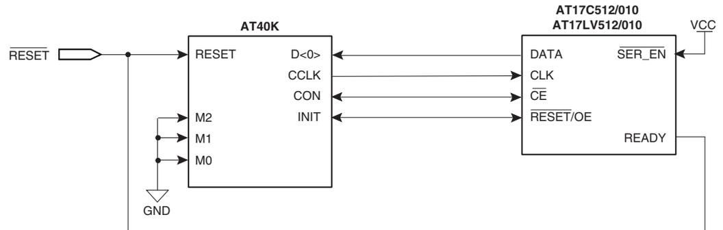
Notes: 1. Use of the READY pin is optional. The READY pin is not available in the 8-pin DPDIP/SOIC package.
