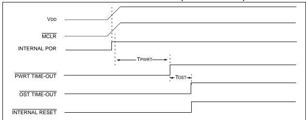
FIGURE 3-4: TIME-OUT SEQUENCE ON POWER-UP (MCLR NOT TIED TO VDD): CASE 1
