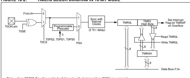
Note: Upon RESET, Timer0 is enabled in 8-bit mode with clock input from T0CKI max. prescale.
