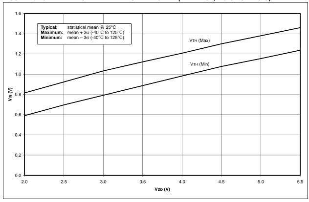
FIGURE 23-27: MINIMUM AND MAXIMUM VIN vs. VDD (I<sup>2</sup>C INPUT, -40°C TO +125°C)
