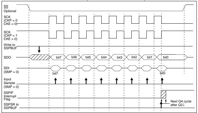
FIGURE 15-6: SPI MODE WAVEFORM (SLAVE MODE WITH CKE = 1)
