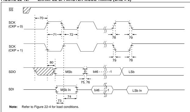
FIGURE 22-12: EXAMPLE SPI MASTER MODE TIMING (CKE = 0)
