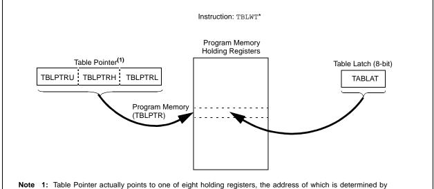
Note 1: Table Pointer actually points to one of eight holding registers, the address of which is determined by TBLPTRL<2:0>. The process for physically writing data to the Program Memory Array is discussed in Section 5.5.
