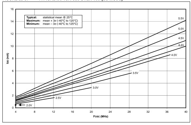
FIGURE 23-10: MAXIMUM IDD vs. Fosc OVER VDD (EC MODE)
