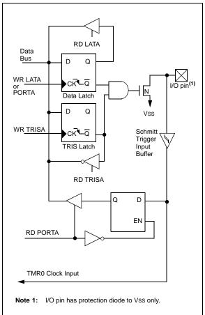
FIGURE 9-3: BLOCK DIAGRAM OF RA6 PIN
