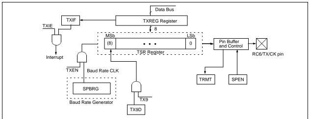
FIGURE 16-2: ASYNCHRONOUS TRANSMISSION
