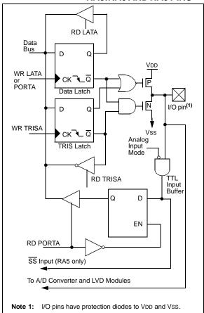
FIGURE 9-2: BLOCK DIAGRAM OF RA4/TOCKI PIN
