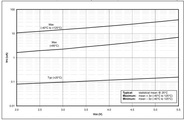
FIGURE 23-16:  $\triangle$ IBOR vs. VDD OVER TEMPERATURE (BOR ENABLED, VBOR = 2.00 - 2.16V)
