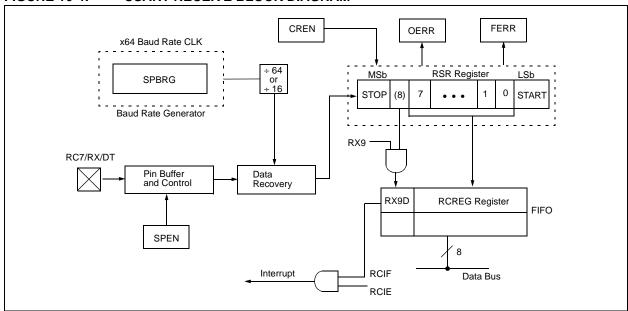
FIGURE 16-5: ASYNCHRONOUS RECEPTION
