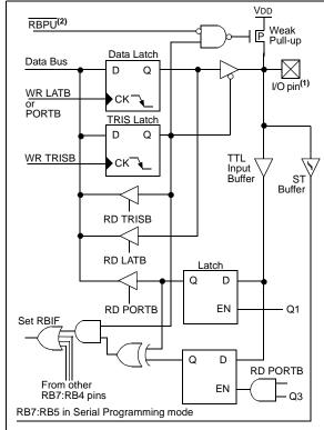
Note 1: I/O pins have diode protection to VDD and Vss.
