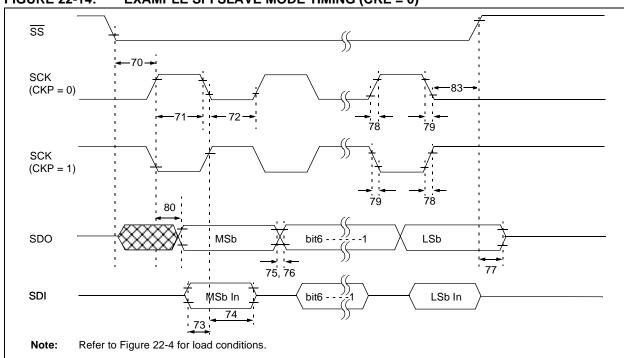
FIGURE 22-14: EXAMPLE SPI SLAVE MODE TIMING (CKE = 0)
