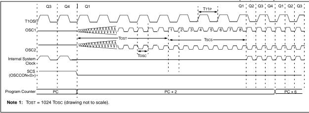
If the main oscillator is configured for HS-PLL mode, an oscillator start-up time (Tost) plus an additional PLL time-out (TPLL) will occur. The PLL time-out is typically 2 ms and allows the PLL to lock to the main oscillator frequency. A timing diagram indicating the transition from the Timer1 oscillator to the main oscillator for HS-PLL mode is shown in Figure 2-10.
