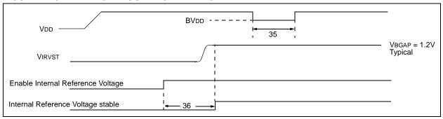
TABLE 22-7: RESET, WATCHDOG TIMER, OSCILLATOR START-UP TIMER, POWER-UP TIMER AND BROWN-OUT RESET REQUIREMENTS
