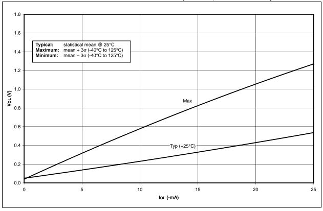
FIGURE 23-24: TYPICAL AND MAXIMUM Vol vs. lol (VDD = 3V, -40°C TO +125°C)
