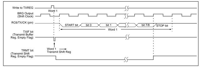
FIGURE 16-3: ASYNCHRONOUS TRANSMISSION (BACK TO BACK)
