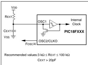
The RCIO Oscillator mode functions like the RC mode, except that the OSC2 pin becomes an additional general purpose I/O pin. The I/O pin becomes bit 6 of PORTA (RA6).
