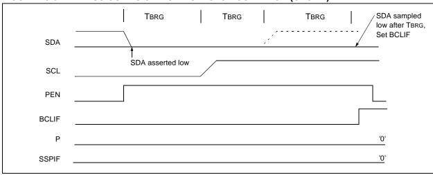
FIGURE 15-32: BUS COLLISION DURING A STOP CONDITION (CASE 2)
