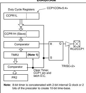
A PWM output (Figure 14-4) has a time-base (period) and a time that the output stays high (duty cycle). The frequency of the PWM is the inverse of the period (1/period).
