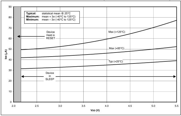
FIGURE 23-17: TYPICAL AND MAXIMUM  $\triangle$ ITMR1 vs. VDD OVER TEMPERATURE (-10°C TO +70°C, TIMER1 WITH OSCILLATOR, XTAL = 32 kHz, C1 AND C2 = 47 pF)
