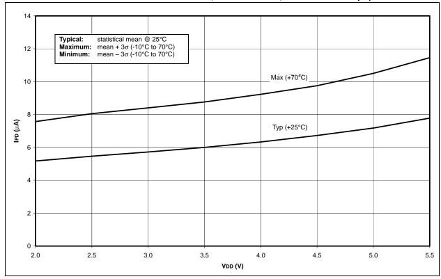
FIGURE 23-18: TYPICAL AND MAXIMUM AIWDT vs. VDD OVER TEMPERATURE (WDT ENABLED)
