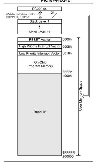
FIGURE 4-2: PROGRAM MEMORY MAP AND STACK FOR PIC18F452/252
