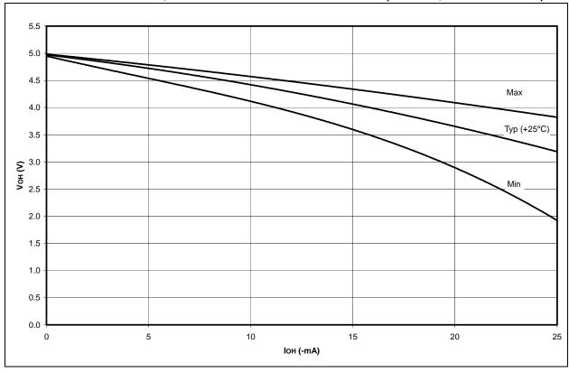
FIGURE 23-22: TYPICAL, MINIMUM AND MAXIMUM VOH vs. IOH (VDD = 3V, -40°C TO +125°C)
