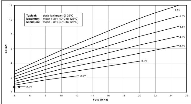
FIGURE 23-3: TYPICAL IDD vs. Fosc OVER VDD (HS/PLL MODE)
