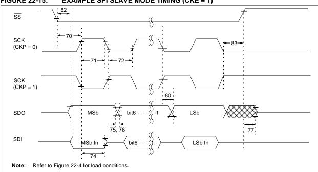
FIGURE 22-15: EXAMPLE SPI SLAVE MODE TIMING (CKE = 1)
