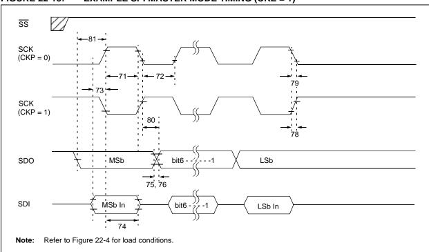
FIGURE 22-13: EXAMPLE SPI MASTER MODE TIMING (CKE = 1)
