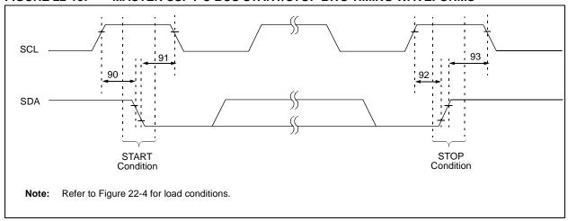
TABLE 22-17: MASTER SSP I<sup>2</sup>C BUS START/STOP BITS REQUIREMENTS
