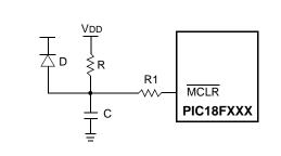
Note 1: External Power-on Reset circuit is required only if the VDD power-up slope is too slow. The diode D helps discharge the capacitor quickly when VDD powers down.
