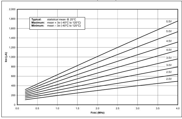
FIGURE 23-6: MAXIMUM IDD vs. Fosc OVER VDD (XT MODE)
