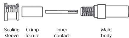
For equipment receptacle: Male contact
