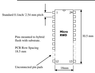
Minimum height occupied by module above host PCB: 6mm +/- 5%
