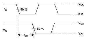
NOTE: All V<sub>I</sub> input pulses are supplied by a generator having the following characteristics:  $t_r$  or  $t_f \le 6$  ns, Pulse Repetition Rate (PRR) = 25 kHz, 50% duty cycle
