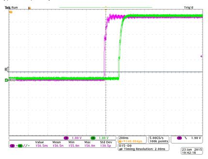
Figure 29. tLOOP Delay Waveform
