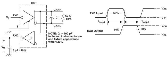
A. All  $V_1$  input pulses are from 0V to  $V_{CC}$  and supplied by a generator having the following characteristics:  $t_r$  or  $t_f \le 6$  ns. Pulse Repetition Rate (PRR) = 125 kHz, 50% duty cycle.
