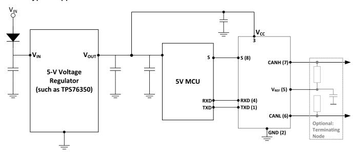
Figure 25. Typical Application Schematic
