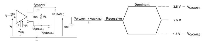
Figure 11. Driver Voltage, Current, and Test Definition
