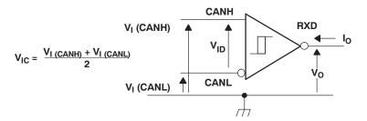
Figure 15. Receiver Voltage and Current Definitions
