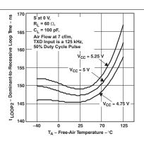
Figure 2. Dominant-to-Recessive Loop Time vs Free-Air Temperature (Across V<sub>CC</sub>)
