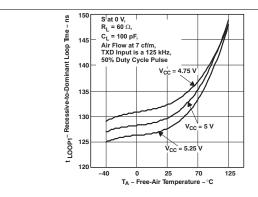
Figure 1. Recessive-to-Dominant Loop Time vs Free-Air Temperature (Across  $V_{CC}$ )
