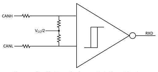
Figure 24. Simplified Recessive Common Mode Bias and Receiver
