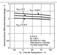
Figure 6. Driver Differential Output Voltage vs Free-Air Temperature (Across V<sub>CC</sub>)
