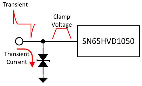
Figure 28. Effect of Transient Voltage Supressor
