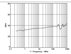
Figure 10. Direct Power Injection (DPI) Response vs Frequency
