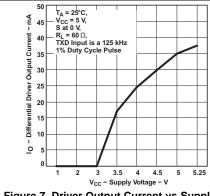
Figure 7. Driver Output Current vs Supply Voltage
