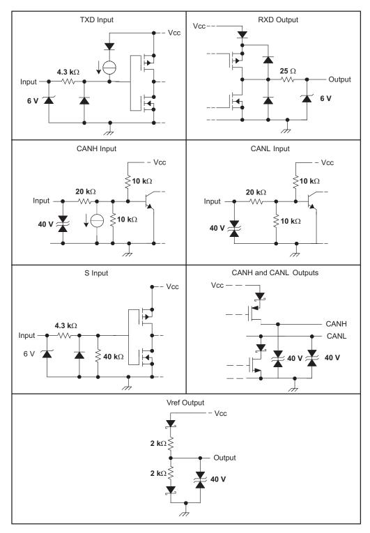
Figure 22. Equivalent Input and Output Schematic Diagrams
