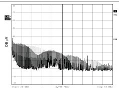
Figure 9. Frequency Spectrum of Common-Mode Emissions
