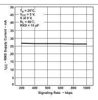
Figure 3. Supply Current (RMS) vs Signaling Rate
