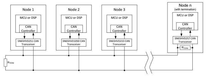
Figure 26. Typical CAN Bus
