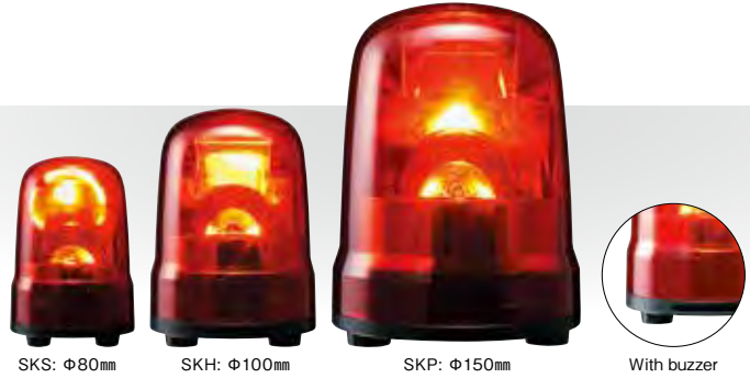
● Use the optional rubber gasket to increase the IP rating from IP23 to IP65. (SKS, SKH only)
