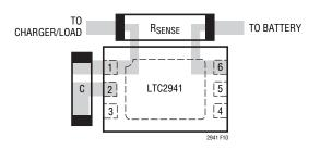
Figure 10. Kelvin Connection on Sense Resistor
