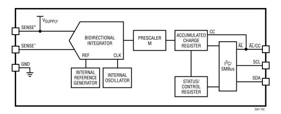
Figure 2. Block Diagram of the LTC2941
