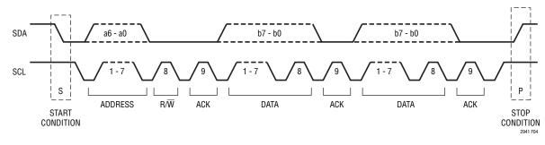
Figure 4. Data Transfer Over I<sup>2</sup>C or SMBus
