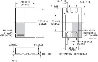
DCB Package 6-Lead Plastic DFN (2mm × 3mm)
