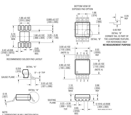
**MS8E** Package 8-Lead Plastic MSOP, Exposed Die Pad
