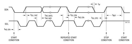
Figure 1. Definition of Timing on I<sup>2</sup>C Bus
