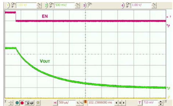
Figure 27. Shutdown, No Load, Output Discharge Enabled
