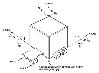
NOTES 1. ACCELERATION  $(a_X,a_Y,a_Z)$  AND ROTATIONAL  $(g_X,g_Y,g_Z)$  ARROWS INDICATE THE DIRECTION OF MOTION THAT PRODUCES A POSITIVE OUTPUT.
