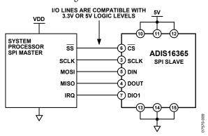
Figure 9. Electrical Connection Diagram
