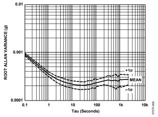
Figure 8. Accelerometer Allan Variance
