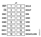
Figure 17. J1Pin Assignments for the ADIS16IMU2/PCBZ
