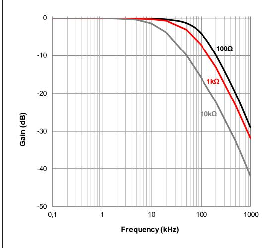
Testcondition:  $I_C = 2$  mA;  $V_{CF} = 2$  V;  $T_A = 25$  °C
