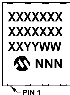
8-Lead DFN-S (6x5x0.9 mm)
