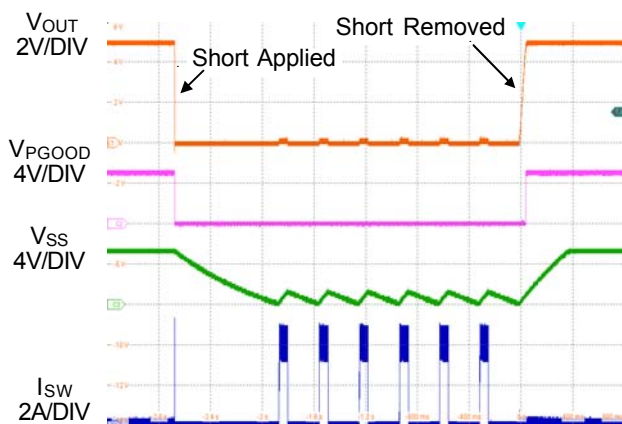
Figure 3. Short Circuit Protection and Recovery
