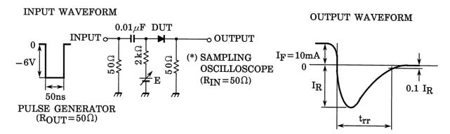
Fig.1 Reverse Recovery Time (trr) Test Circuit
