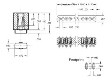
**Description:** Interconnect Socket Surface Mount Socket Accepts .015" - .022" (0,38 - 0,559 mm) dia leads Single Row Surface Mount **Plating Code:** Shell Plating:
